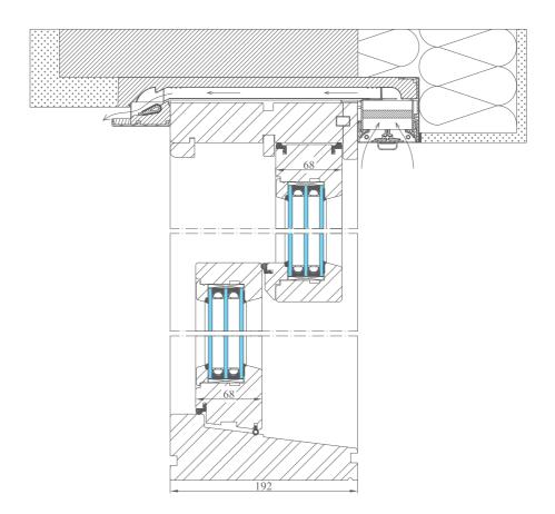
ventilator with sound insulation 42dB and particulate filter PM10 – 99%; PM2,5 – 80% triple glazed unit Ug=0,7W/m2/K with argon gas or Uw=0,4W/m2/K with krypton gas option with acoustic glazing unit Rw=43dB timber: high-quality glued-laminated timber pine, meranti sash depth: 68mm paint system – Teknos
